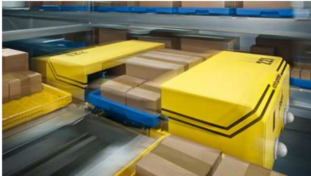
psb Shuttle system vario.sprinter in operation (picture by psb intralogistics GmbH)
