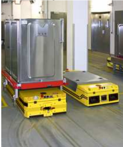
With the modernization, all AGVs were converted to WLAN (on the right, a carobot vehicle of the first generation, with infrared technology; on the left a vehicle with WLAN)
