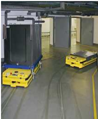
Each AGV can carry each container; thus, empty runs are reduced to a minimum
